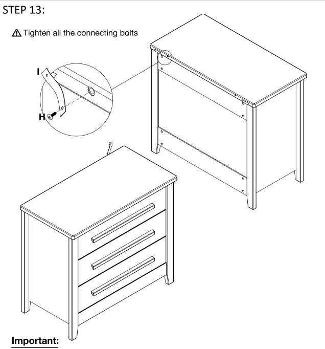
The assembled furniture must be placed adjacent to the wall and fixed to the wall using the appropriate screw for that wall type. If you are in any doubt about the correct type of fitting to use, please seek professional advice.
